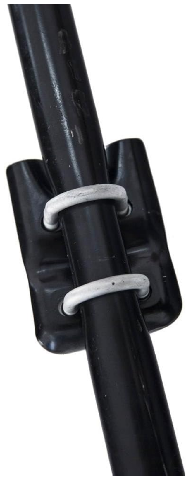
Figure 6.1: Detail of a clamp and bushing on a steering rod. Ensure all clamps and fasteners are secure and free from corrosion during maintenance checks.
