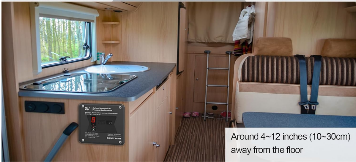
Image: The Leakbee R503 detector mounted inside an RV, demonstrating its recommended placement between 4-12 inches from the floor.
