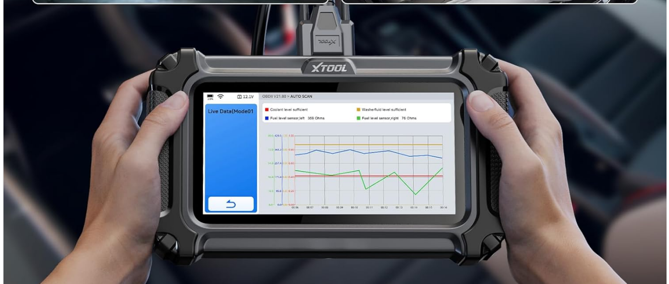
The XTOOL D5S displaying live data streams for various vehicle parameters.
