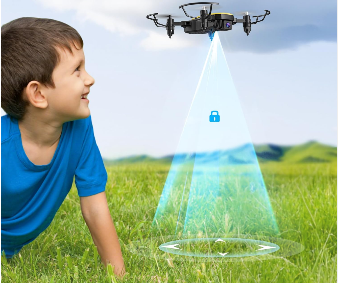
Figure 4: Optical Flow Positioning for stable hovering.
