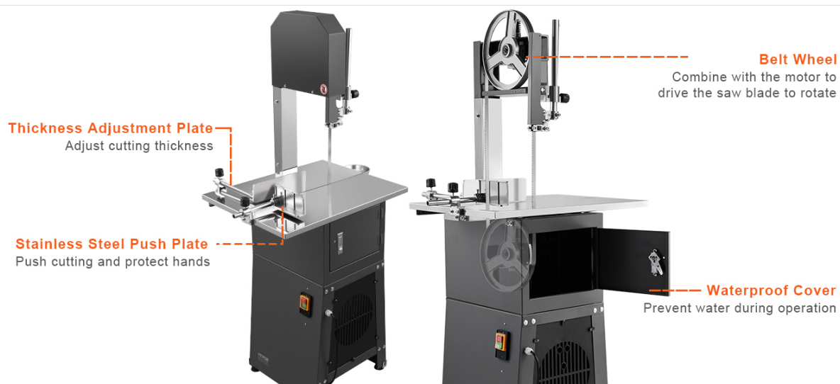
Figure 5.5: Key safety features of the bandsaw.
