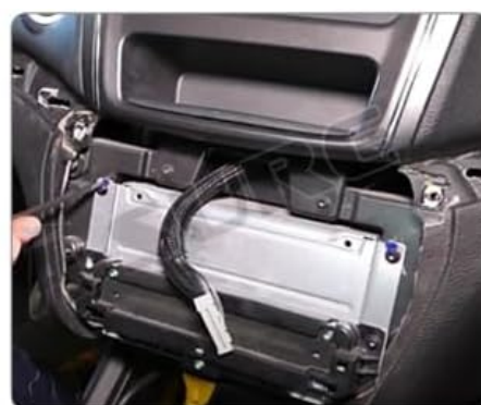
The right OEM connectors are in the silver unit behind the A/C Control Panel
