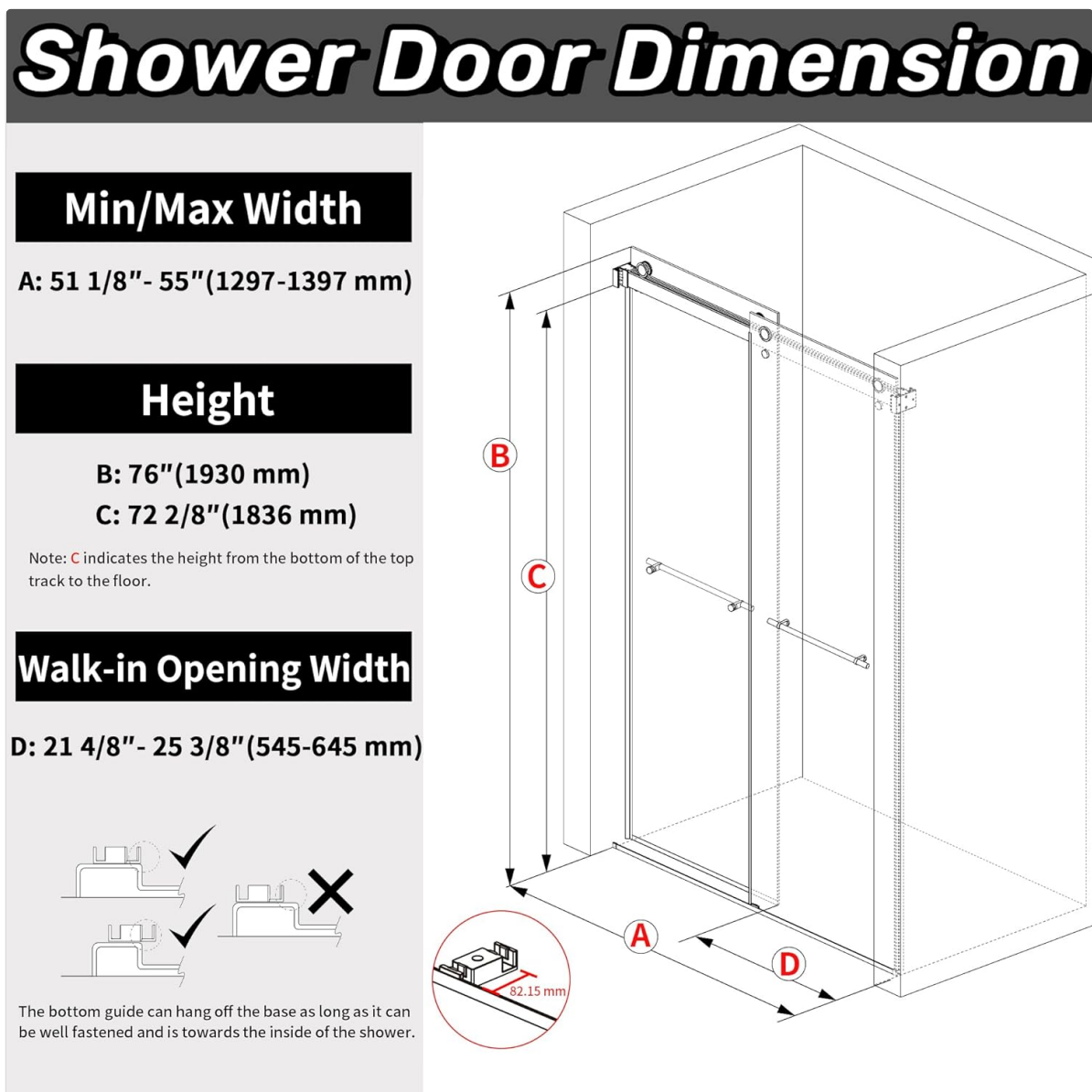
Figure 3: Measuring the shower opening.
