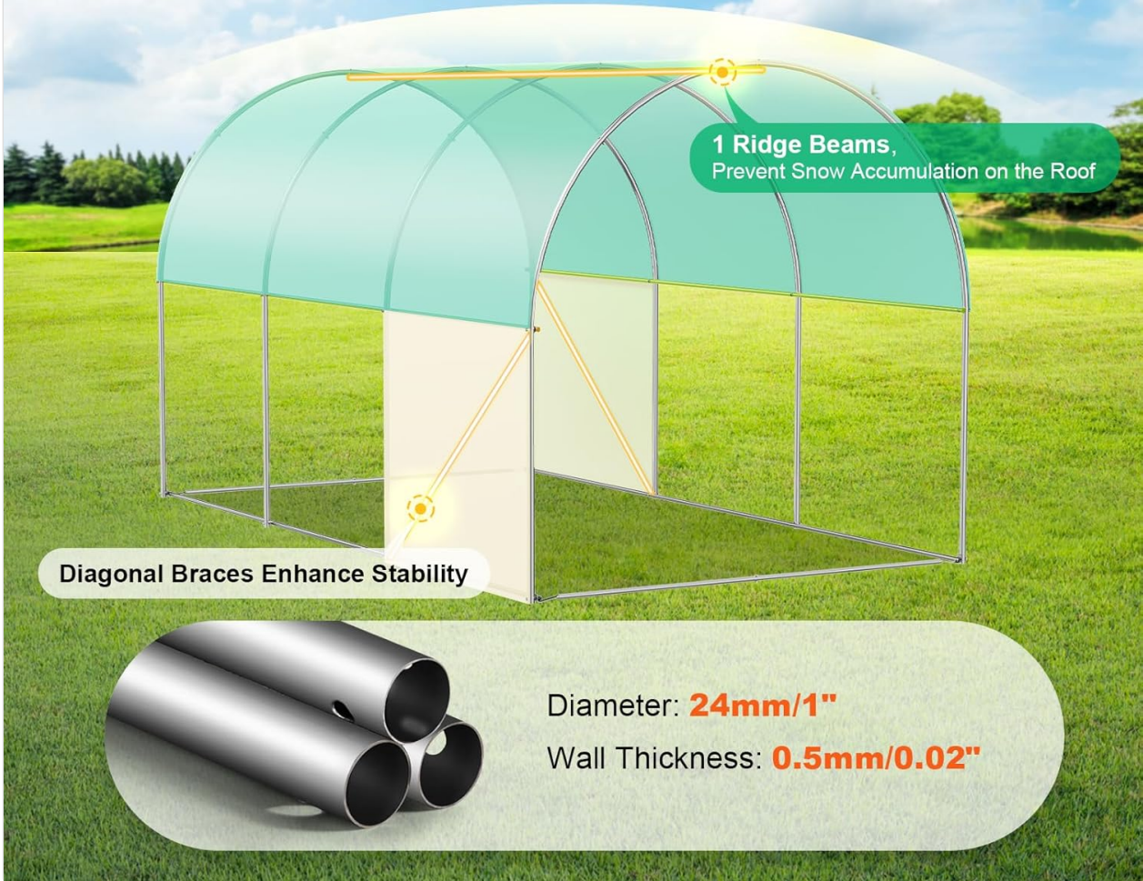
Figure 2.2: Illustration of the greenhouse's sturdy galvanized pipe frame, highlighting the 1-inch diameter and 0.02-inch wall thickness, along with diagonal braces for enhanced stability.
