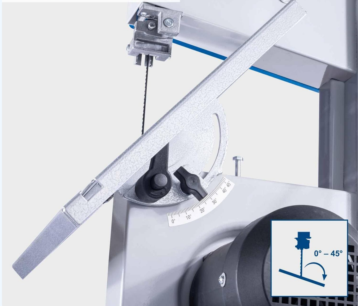
Figure 5.3: The continuously tiltable saw table of the HBS25, allowing for easy and quick implementation of angle cuts up to 45 degrees. This feature is essential for miter cuts.
