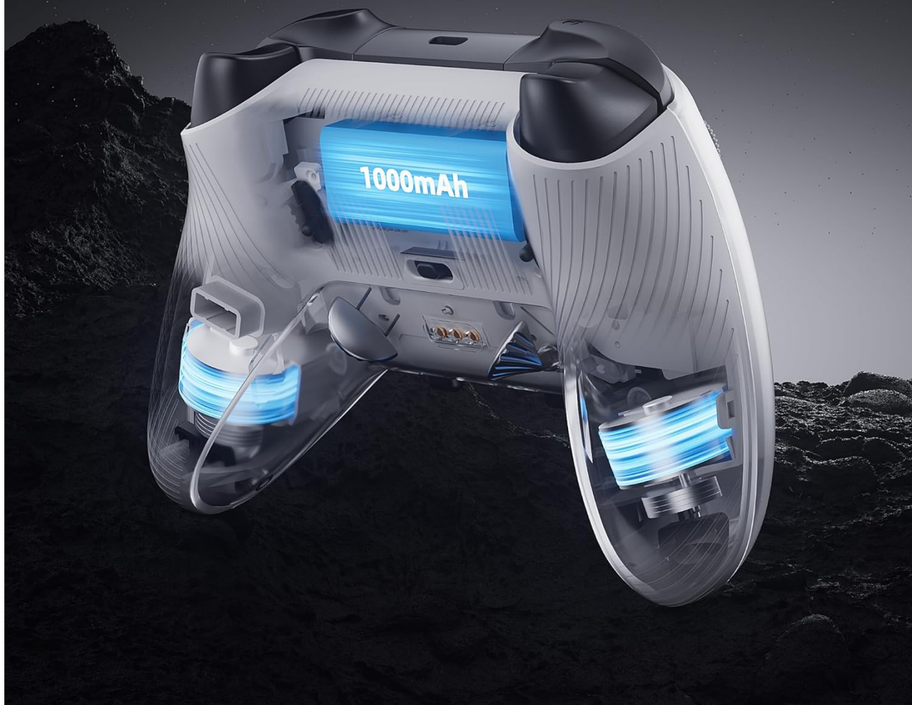
Image: An internal view of the Mytrix Pro PC Controller, highlighting the asymmetrical rotor motors responsible for providing adjustable vibration feedback.
