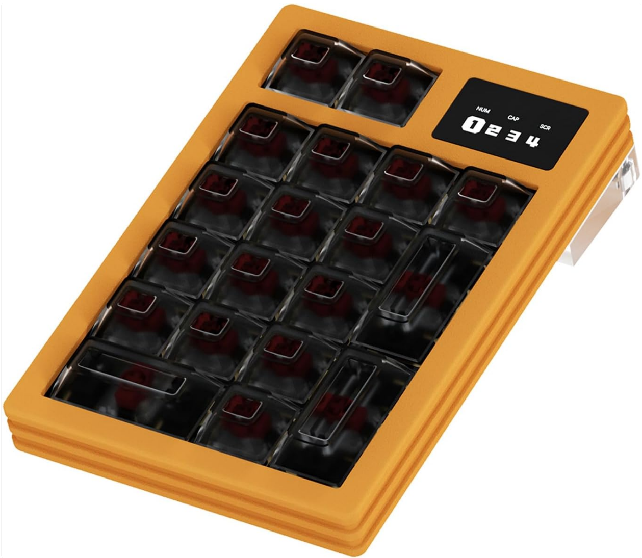
Image: The NLOFIN 19-Key Programmable Mechanical Keypad in yellow, showcasing its compact design and OLED screen.
