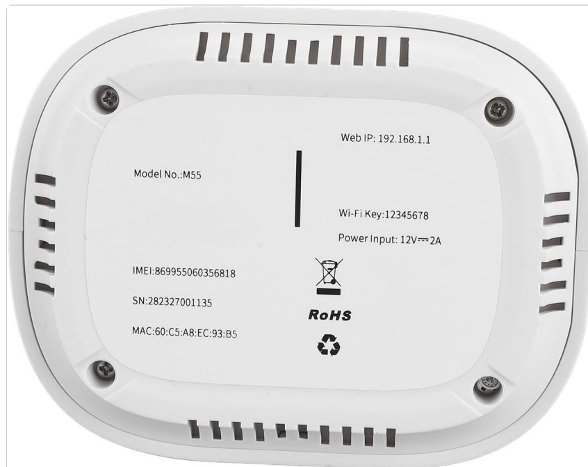
Image: The bottom label of the 5G CPE Router, displaying important information such as Model No.: M55, Web IP: 192.168.1.1, and Wi-Fi Key: 12345678.
