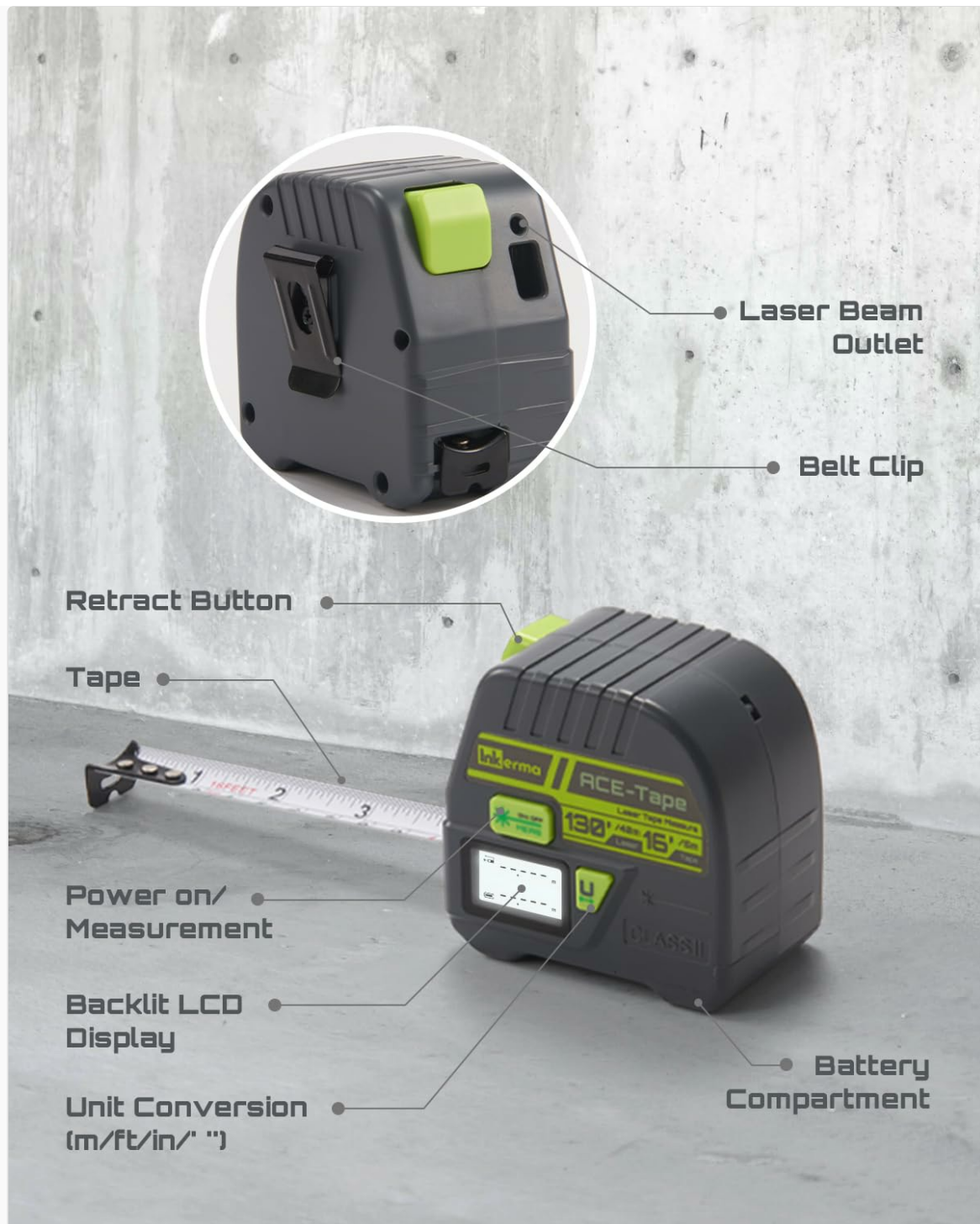
Image 4.1: Key components of the Inkerma Tape-TX1.
