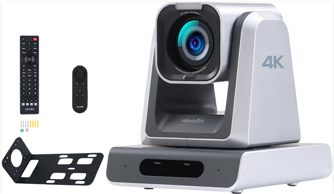
Figure 4.1: Front view of the Zowietek 4K PTZ Camera. Shows the camera lens, the 4K branding, and the base with Power and Status indicators.
