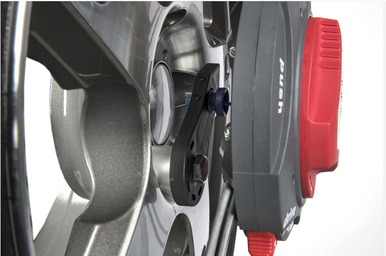
Image: Close-up view of the central attachment mechanism of the pewag RSC 850 SERVOSTAR, showing how it connects to the wheel's lug nut or bolt.
