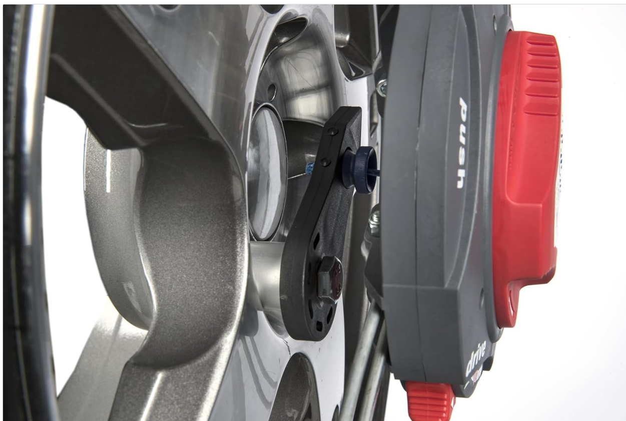
Figure 2.1: Detailed view of the Servostar attachment mechanism connecting to a vehicle's lug nut. This shows the secure, external connection point.
