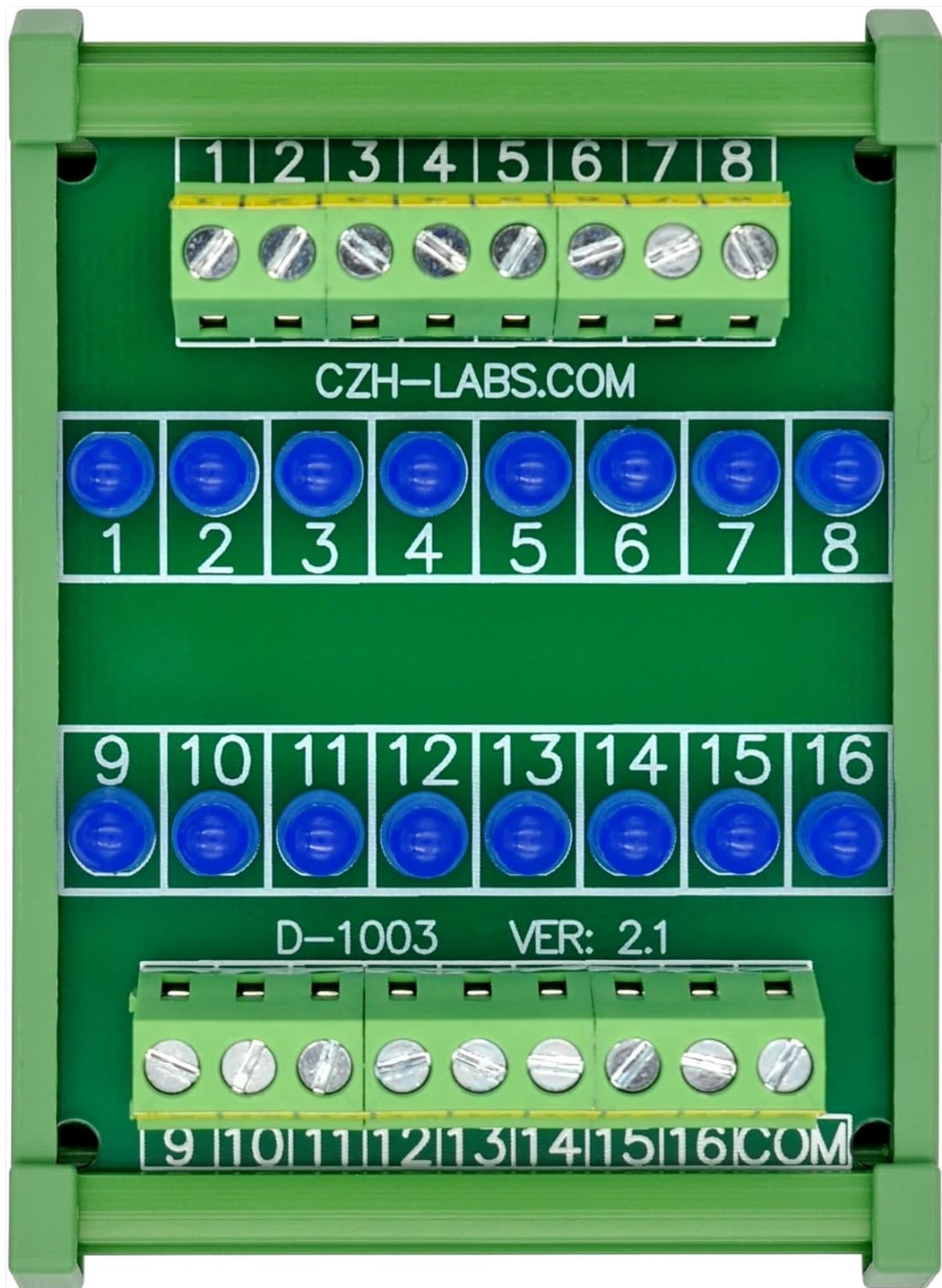
Figure 1: Top-down view of the 16-LED indicator module, showing the LED array and terminal blocks.
