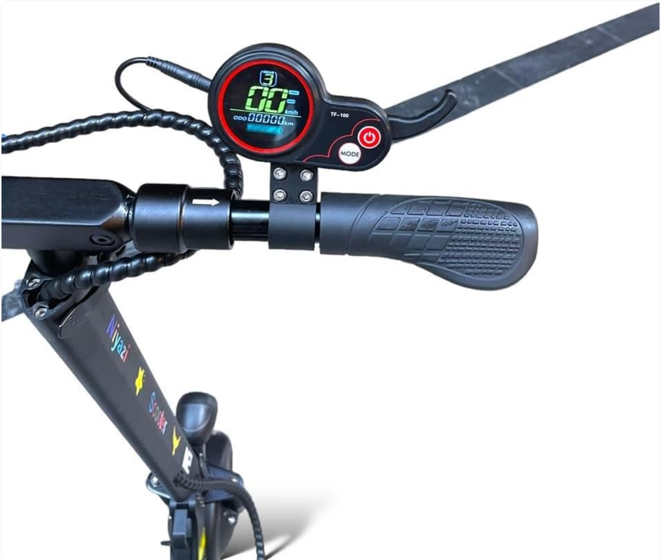
Image: A close-up of the digital display and handlebar controls, including the power button and mode button, on the Monster Mini M2 Electric Scooter.
