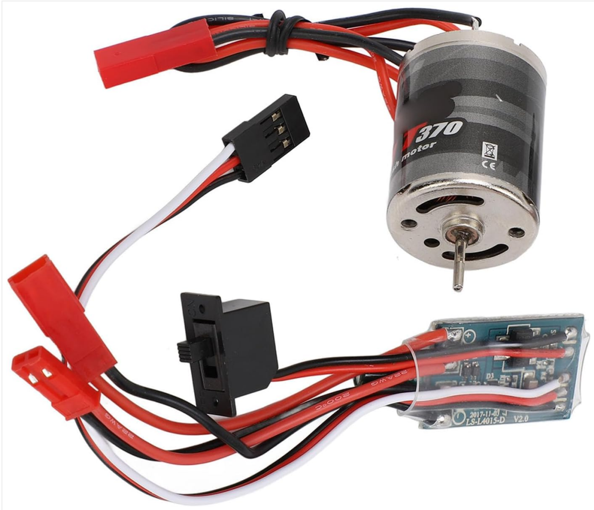
Image 3: A detailed view of the ESC and motor, showing the JST power connector, motor wires, and receiver signal cable.
