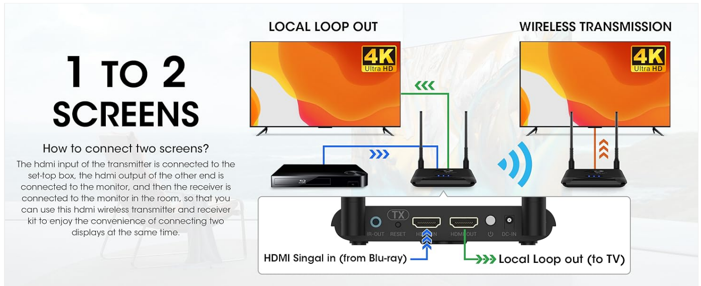
Image 5.1: Connection diagram for using the local loop out feature, allowing simultaneous display on a local monitor and a wirelessly connected TV.
