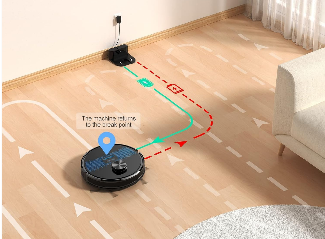
Image: Diagram illustrating the robot vacuum's ability to return to its charging base when the battery is low and then resume cleaning from the exact spot it left off.
