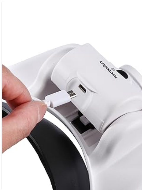
Figure 4: Illustrates the USB charging port and connection.
