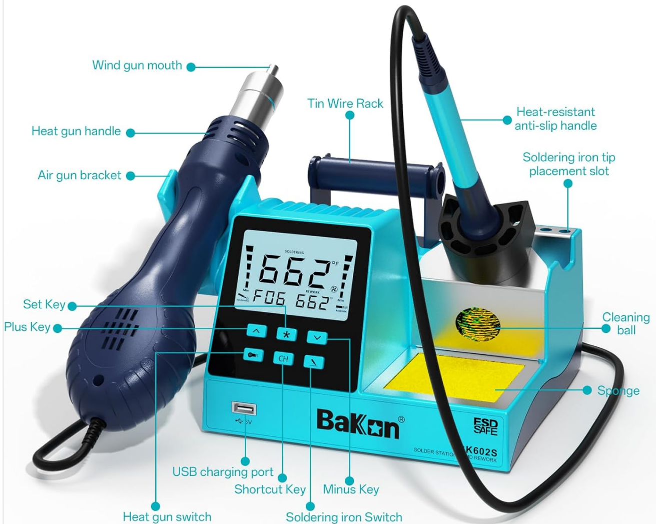
Figure 3.2: Detailed view of the BK602S components and controls.
