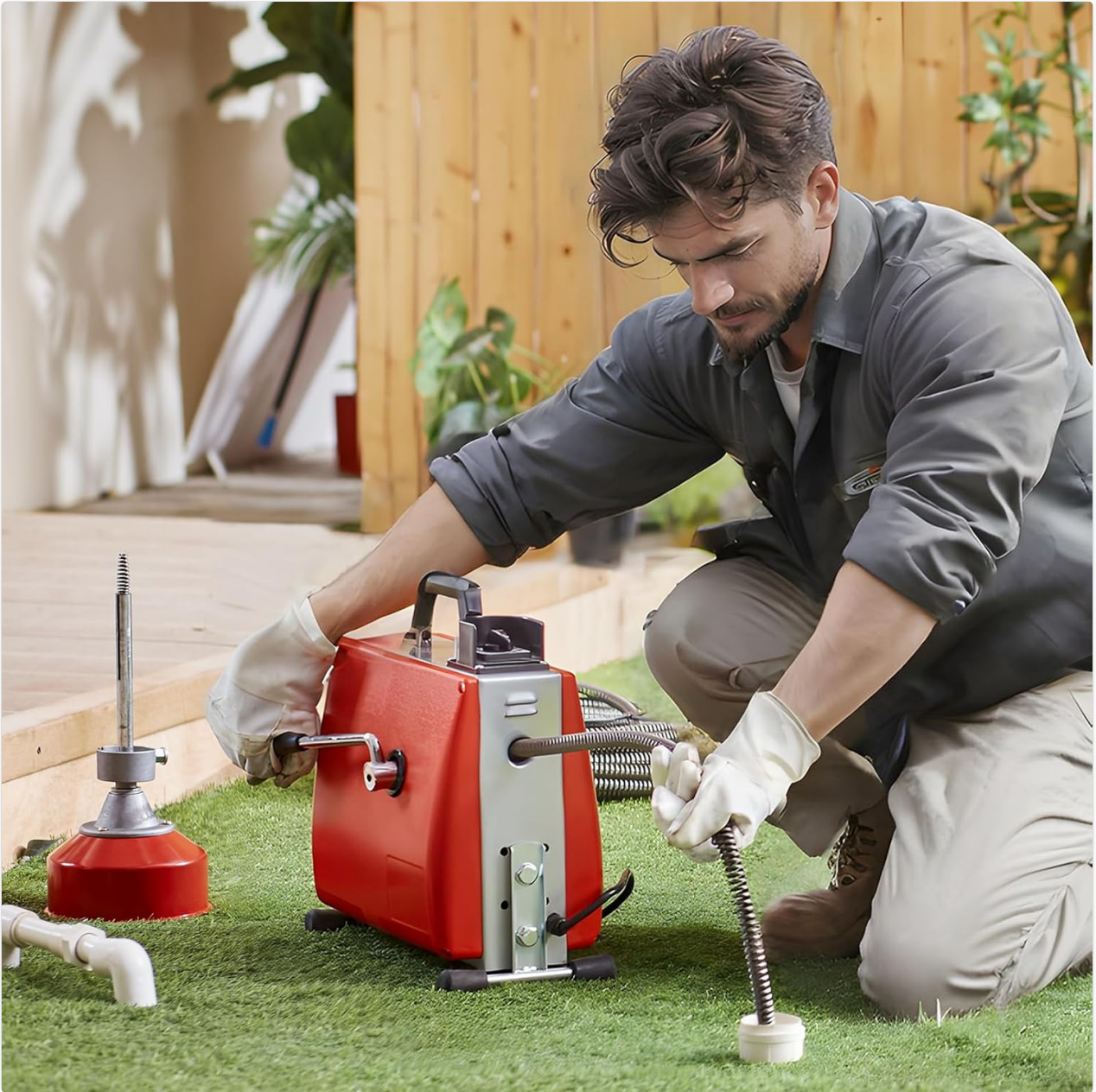
Figure 5.1: Operating the drain cleaner machine.
