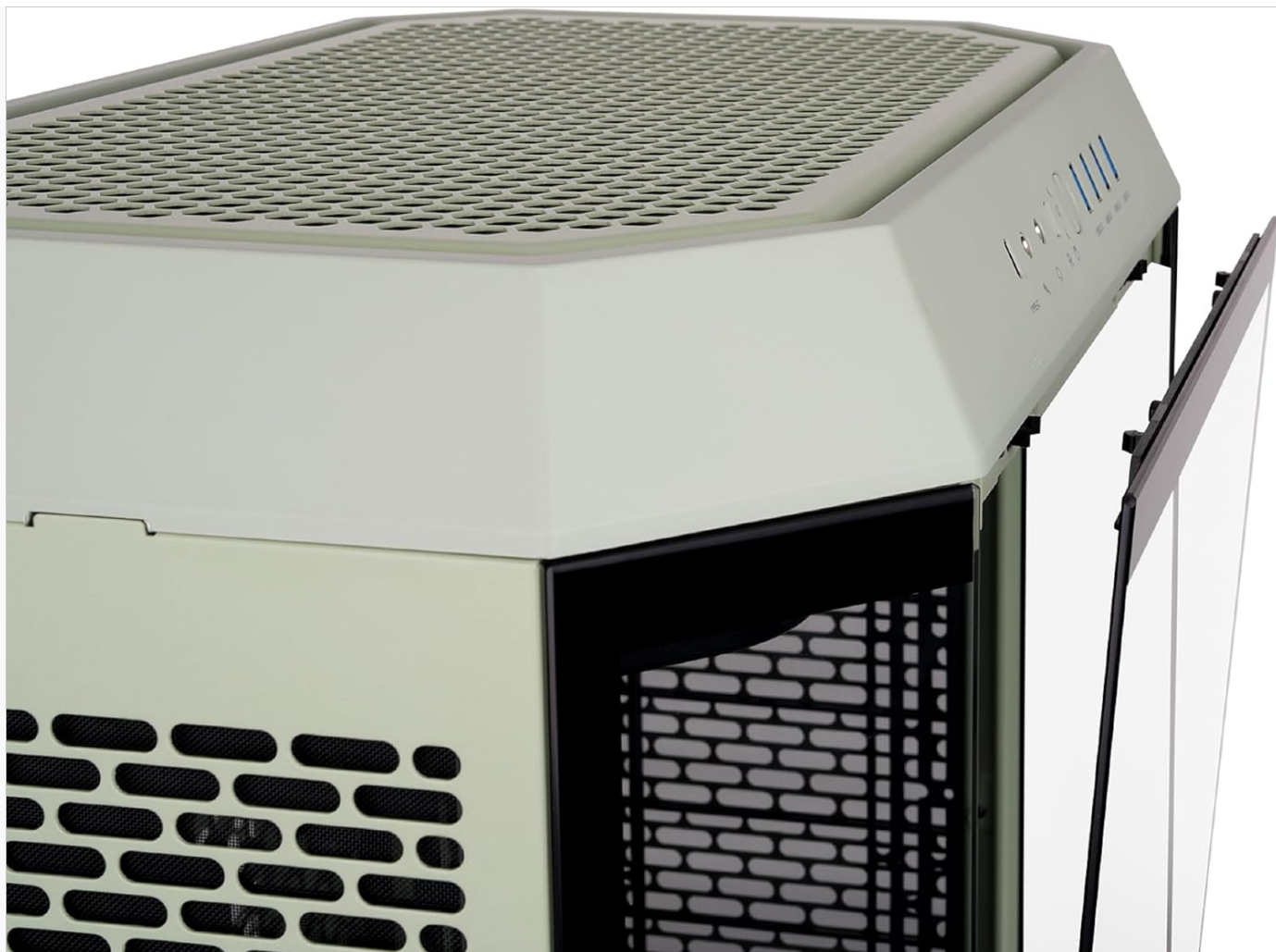
Image 4.1: Top panel removed for access.
