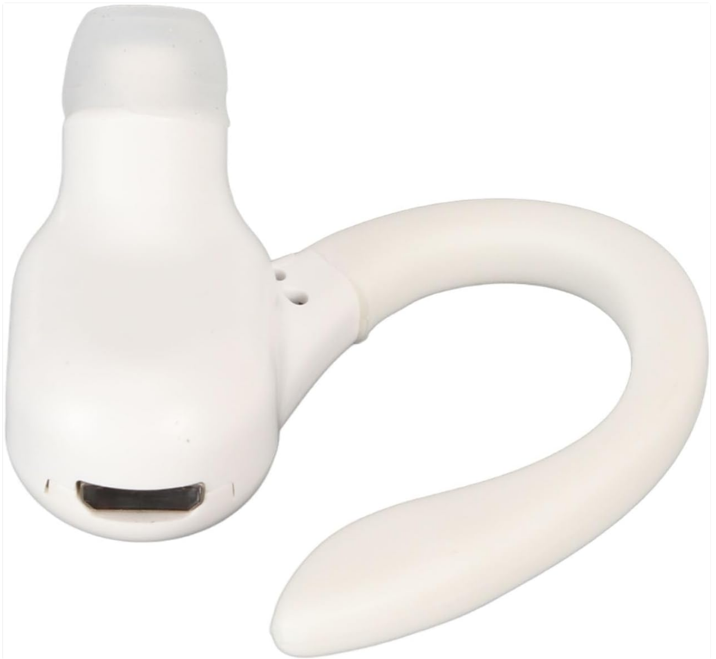
Figure 3: Bottom view of the headset, clearly showing the charging port for power input.
