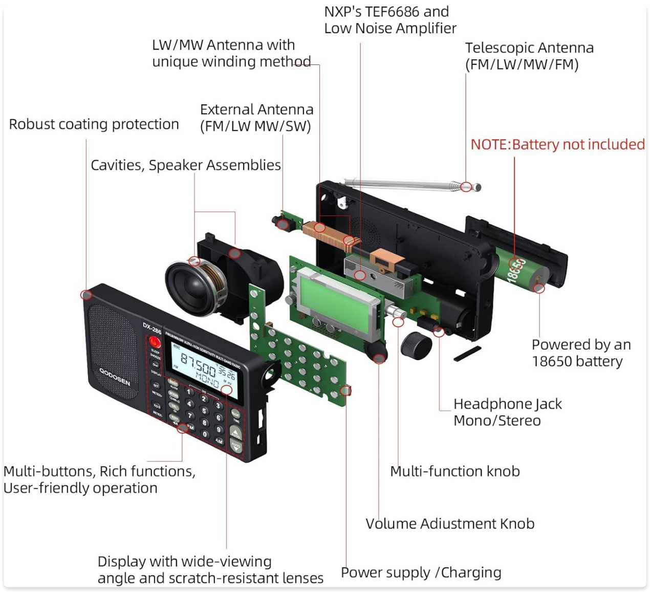
Figure 2.2: Internal Components and Design
