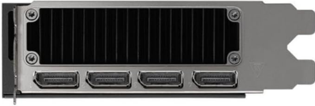
Figure 2.3: Rear view of the NVIDIA RTX 5000 Ada Generation GPU, displaying the multiple DisplayPort outputs for multi-monitor setups.
