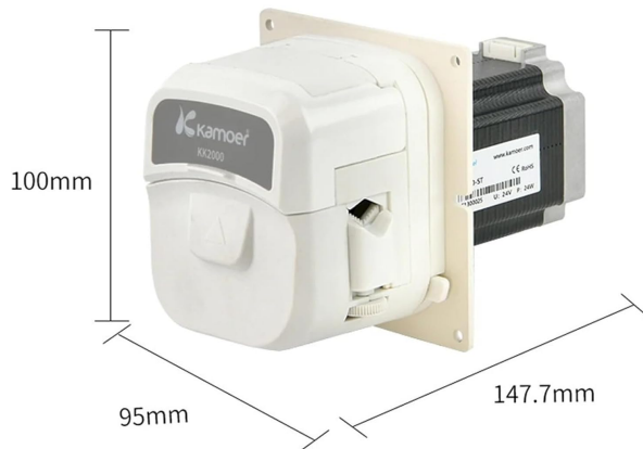
Figure 2: KK2000 Pump with key specifications. This image highlights the pump's flow rate range (700-2000ml/min), accuracy ( \pm 10\% ), optional Modbus driver board, 24W 24V stepper motor, and compatible tubing types (17#, 18# Silicone, BPT).
