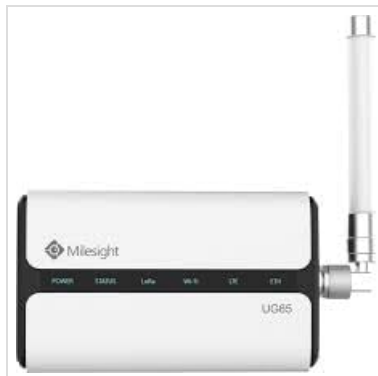
Image 1.1: Front view of the Milesight UG56-868M LoRaWAN Gateway. The device is a compact, rectangular unit with a white and black casing. It features LED indicators for POWER, STATUS, LoRa, Wi-Fi, and ETH, along with the Milesight logo and model number UG56. An antenna is connected to the right side.
