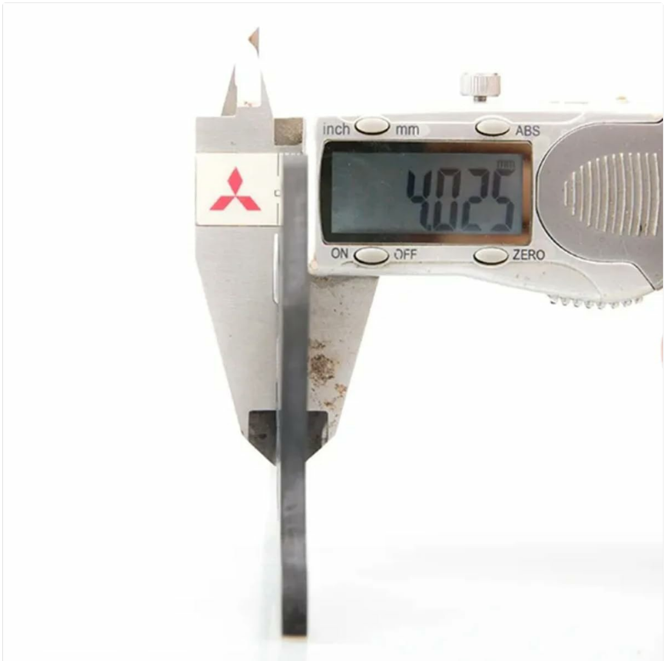
Figure 3.2: Measurement of the 4.0mm 3K real carbon fiber chassis thickness.
