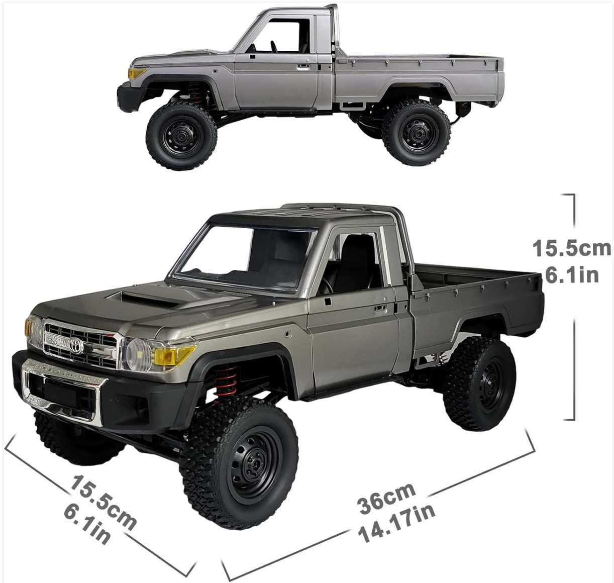
Figure 7.1: Dimensions of the Skymaker MN82PRO RC Truck.
