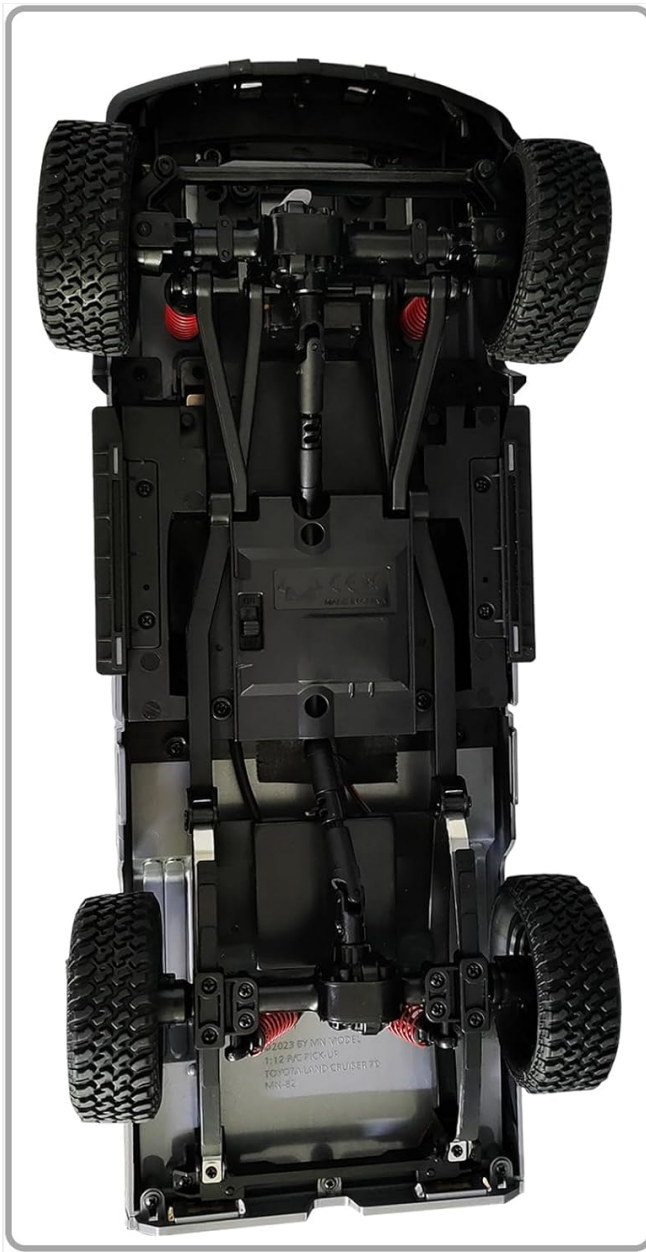
Figure 5.1: Underside of the MN82PRO, highlighting the metal upgrade parts for improved durability and performance.
