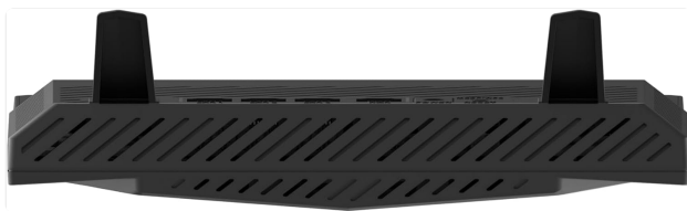
Figure 3.3: Top view of the H3C Magic NX15 router, highlighting the ventilation design for heat dissipation.
