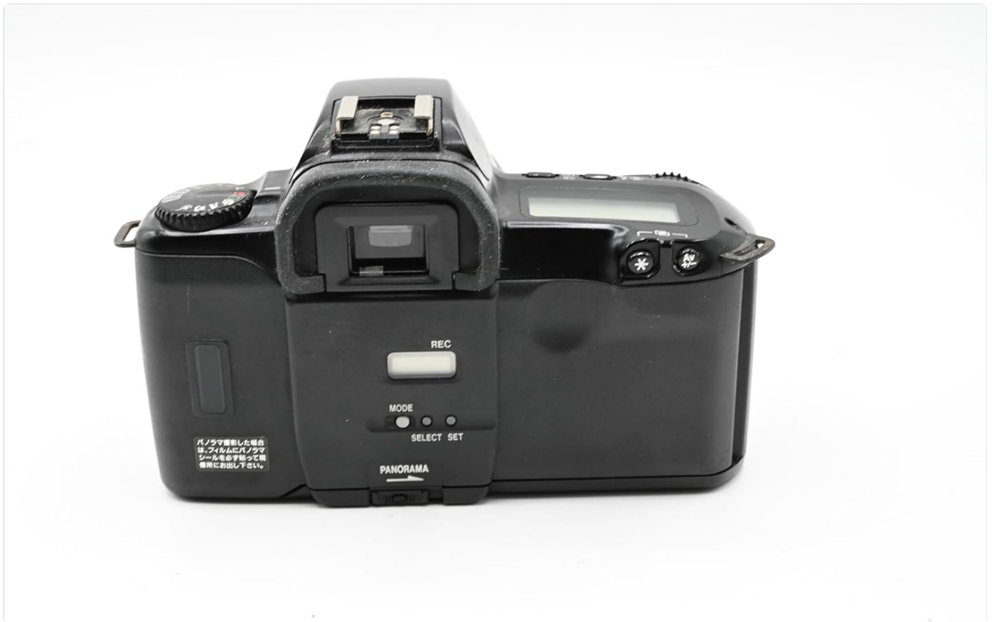
Figure 3: Rear view of the Canon EOS Kiss Panorama camera, displaying the LCD screen, viewfinder, and various control buttons for settings like mode and select/set.
