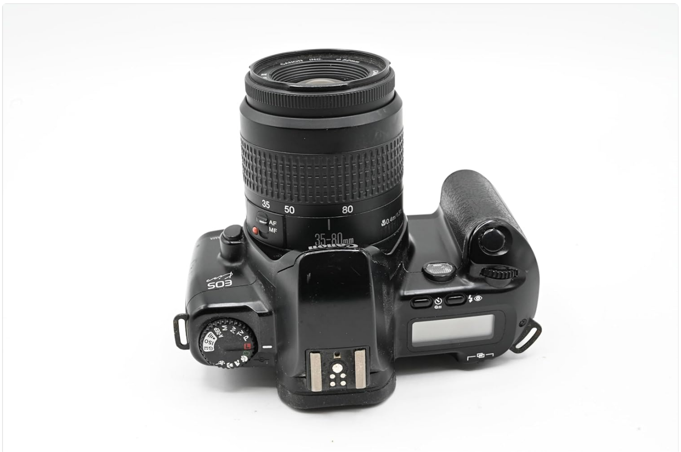
Figure 2: Top view of the Canon EOS Kiss Panorama camera, illustrating the mode dial, shutter button, and other top-mounted controls.
