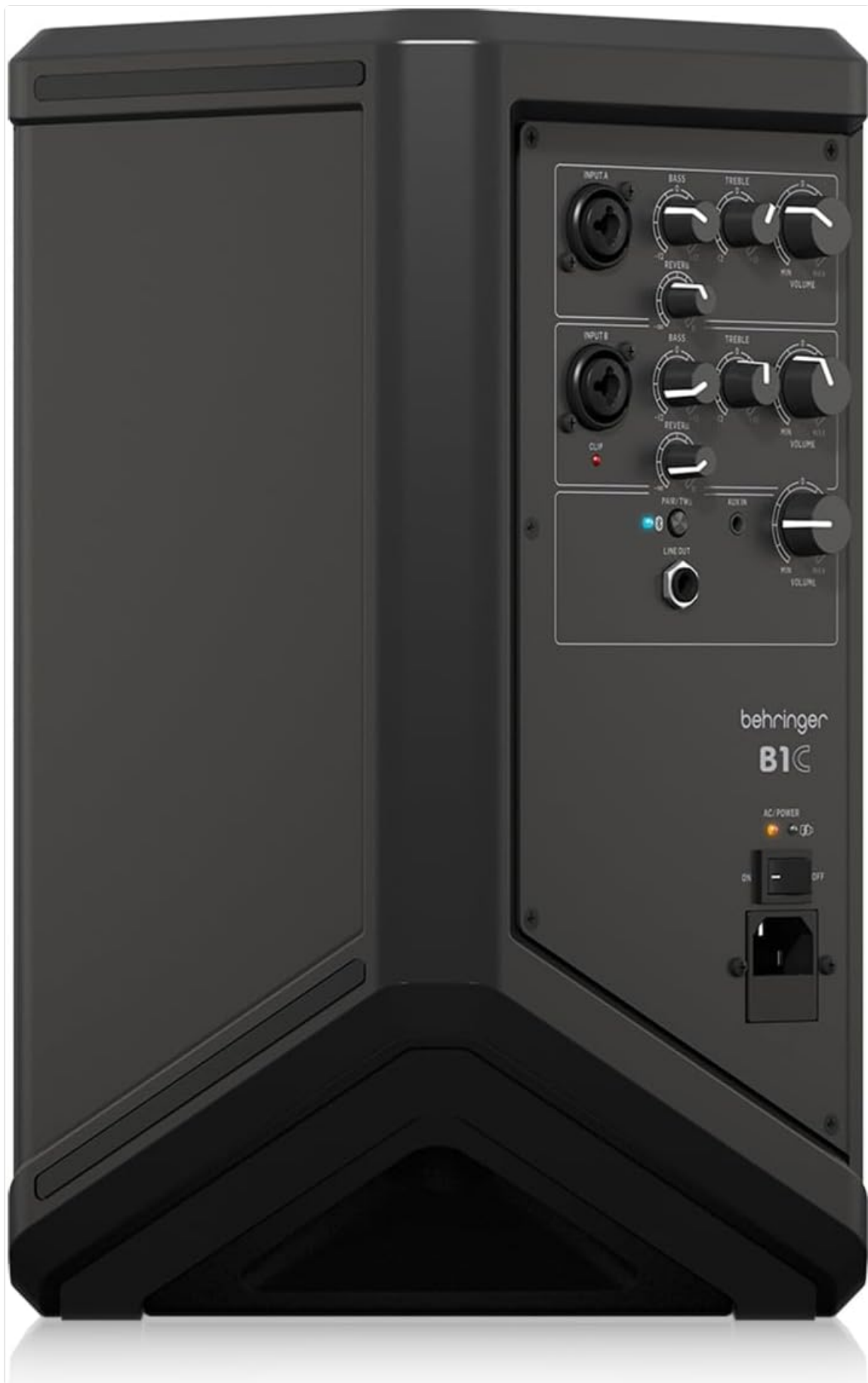
Figure 2: Rear Control Panel Overview
