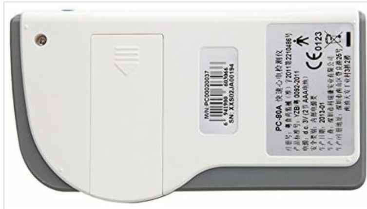
Image 5.1: Rear view of the PC-80A monitor, indicating the battery compartment location.
