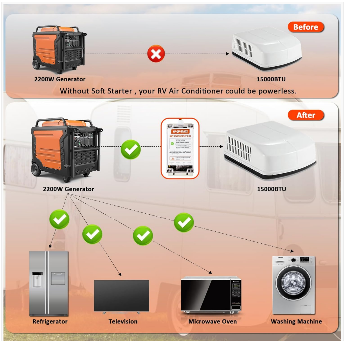
Figure 5.3: Visual comparison demonstrating the ability to power a 15,000 BTU AC and other appliances with a 2200W generator after installing the soft start kit.
