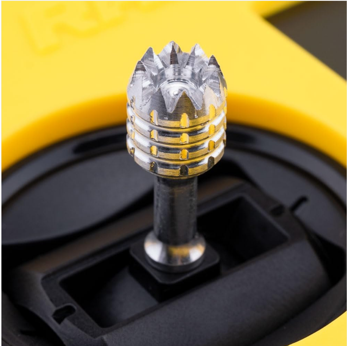
Figure 3.3: Close-up of a Hall effect gimbal.
