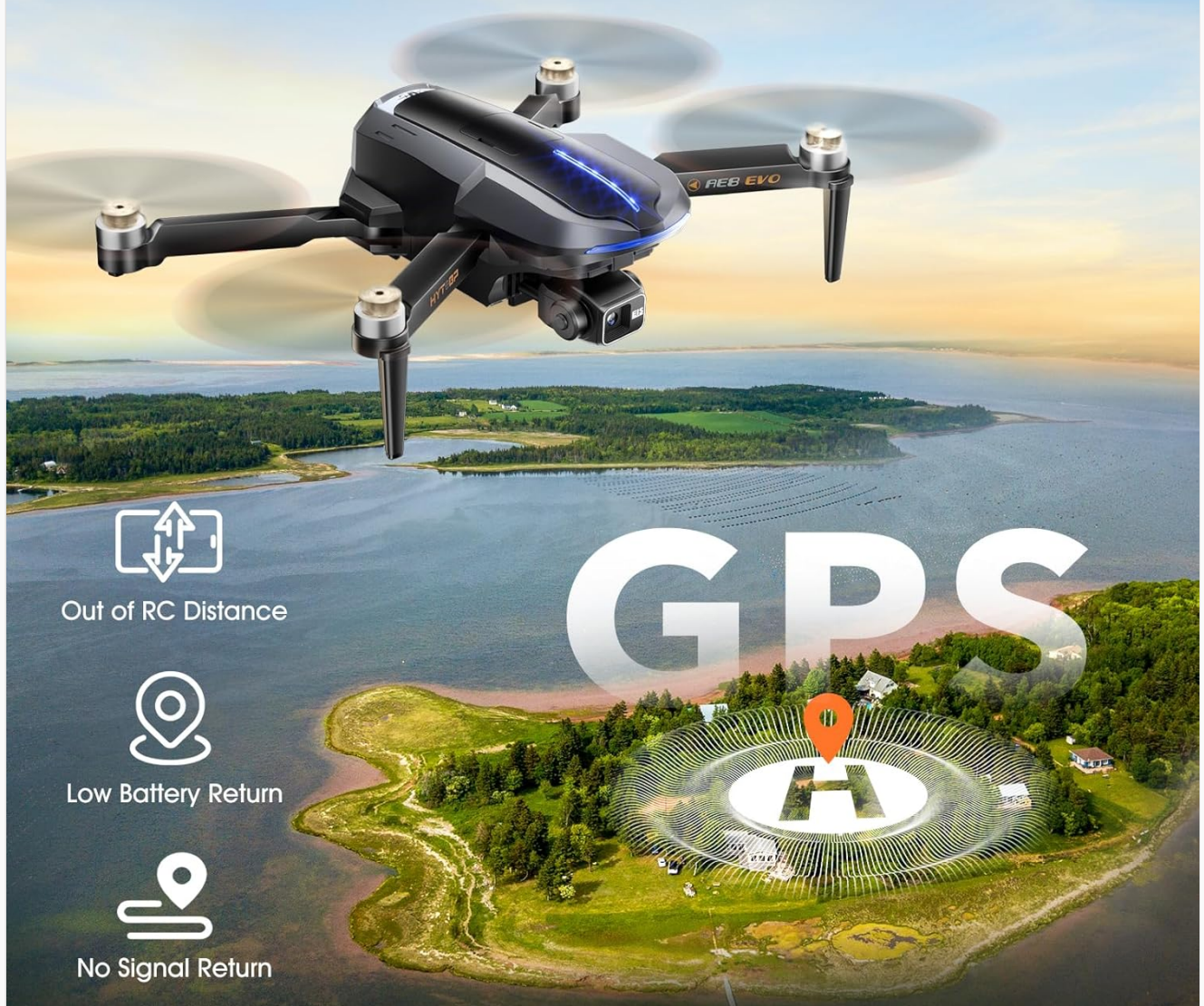
Image 5: The HYTOBP AE8 drone illustrating its GPS intelligent auto-location and return capabilities, which activate in scenarios such as being out of remote control distance, low battery, or signal loss, guiding the drone back to its home point.
