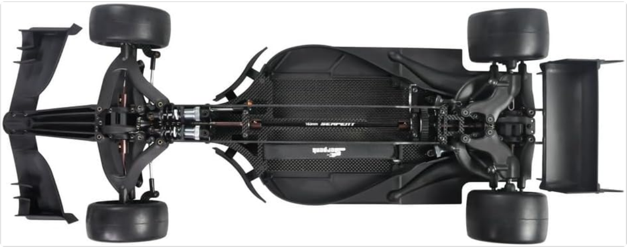
Image: A top-down view of the Serpent F190 chassis, highlighting the central drivetrain and suspension arms.
