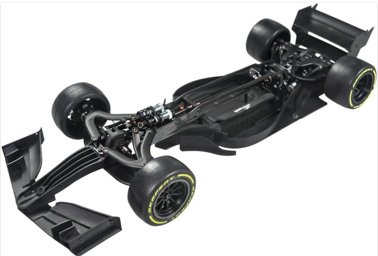
Image: An assembled Serpent F190 chassis, showcasing the carbon fiber structure, suspension components, and drivetrain layout.
