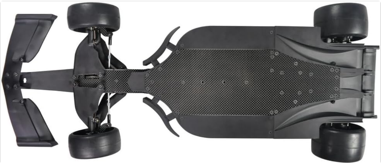
Image: The underside of the Serpent F190 chassis, showing the flat carbon fiber base and protective elements.
