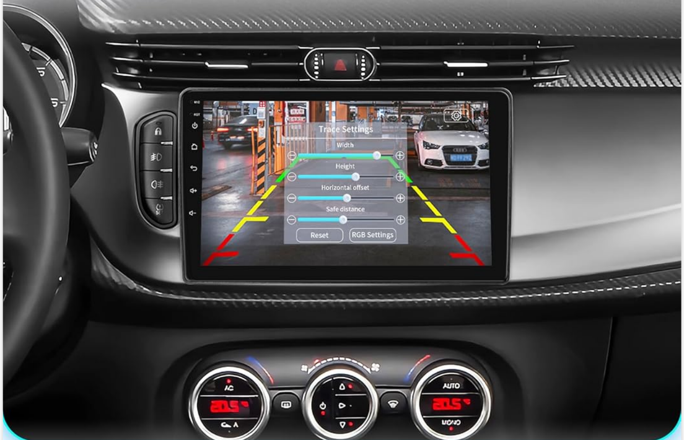
Image 4.10: Rear View System display with adjustable parking guidelines.
