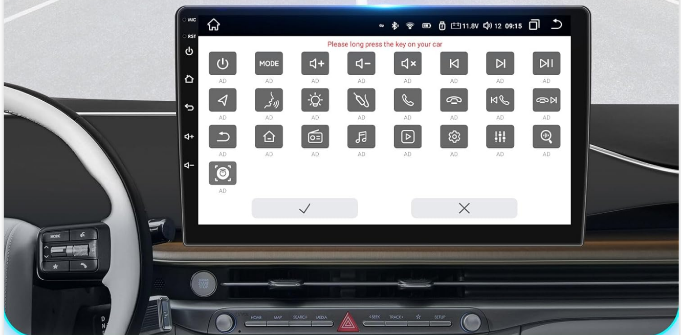
Image 4.9: Steering Wheel Control configuration screen.
