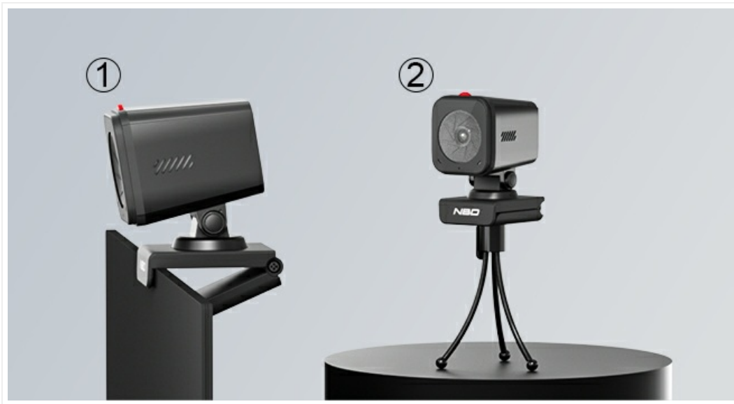
Image: The webcam shown in two mounting configurations: (1) clipped onto a monitor and (2) attached to a tripod, demonstrating its flexible placement options.
