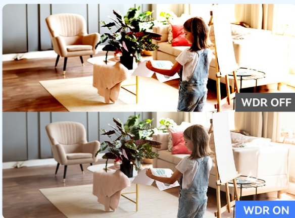
Image: A split image showing a room scene with "WDR OFF" (top, with harsh shadows/highlights) and "WDR ON" (bottom, with balanced exposure), demonstrating the effect of Wide Dynamic Range.
