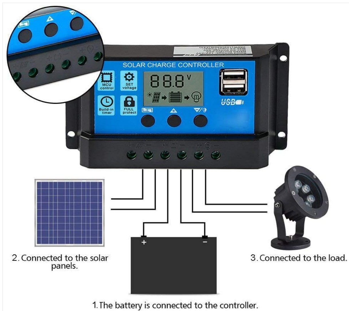
Figure 1: Connection diagram showing the battery, solar panel, and load connected to the solar charge controller. The battery is connected first, followed by the solar panels, and then the load.
