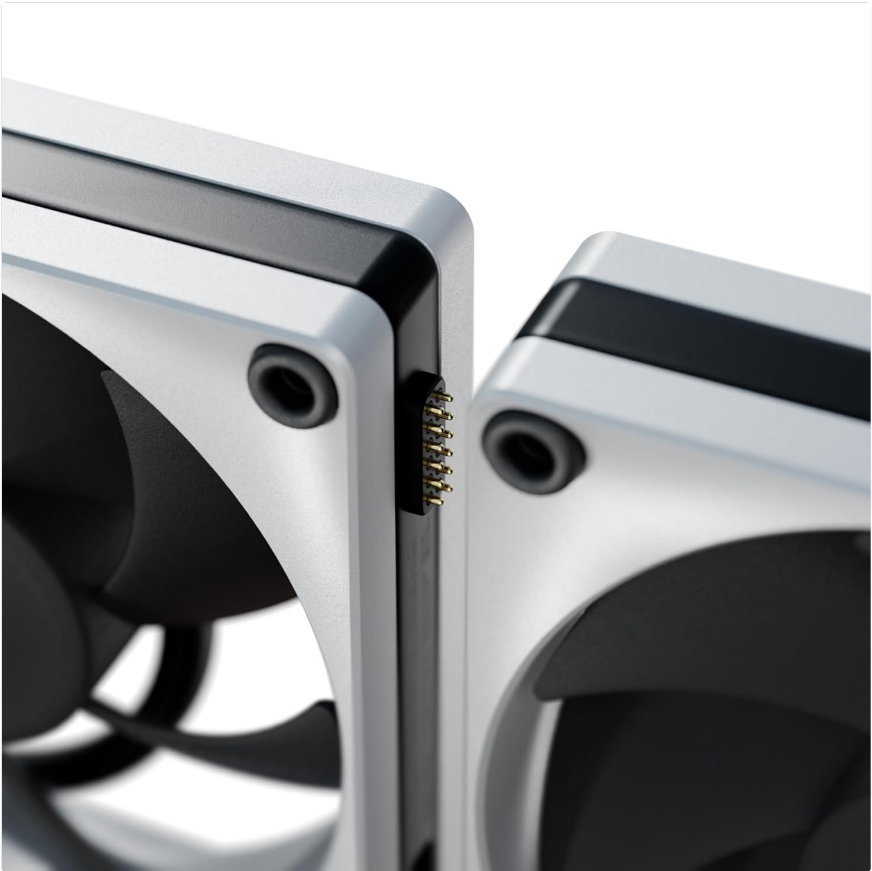
Figure 5: Two FP12 fans connecting via their magnetic Nexus Link pins for sequential power and data transfer.
