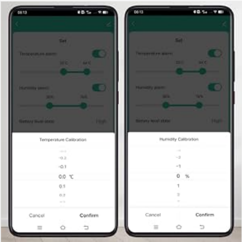
Image: A smartphone screen displaying the app's calibration options for both temperature and humidity, allowing for fine-tuning of readings.
