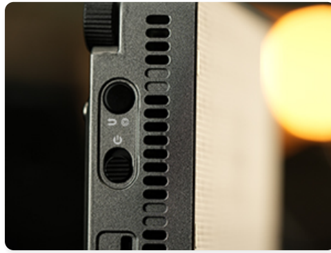
Figure 5.1: Side view of the Amaran Ace 25c, highlighting the power switch and USB-C port.
