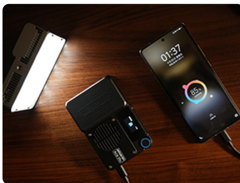
Figure 3.3: The Amaran Ace 25c can charge other devices via its USB-C port.
