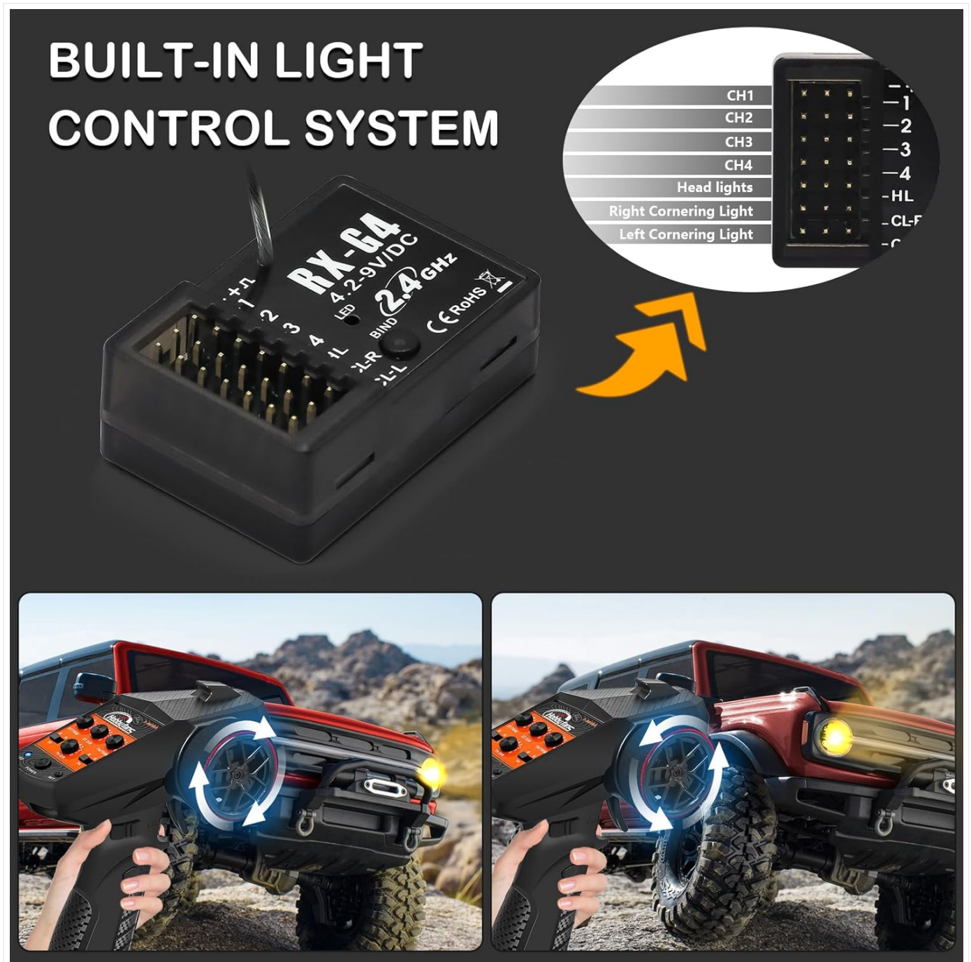
Figure 3: RX-G4 Receiver Ports and Indicators.
