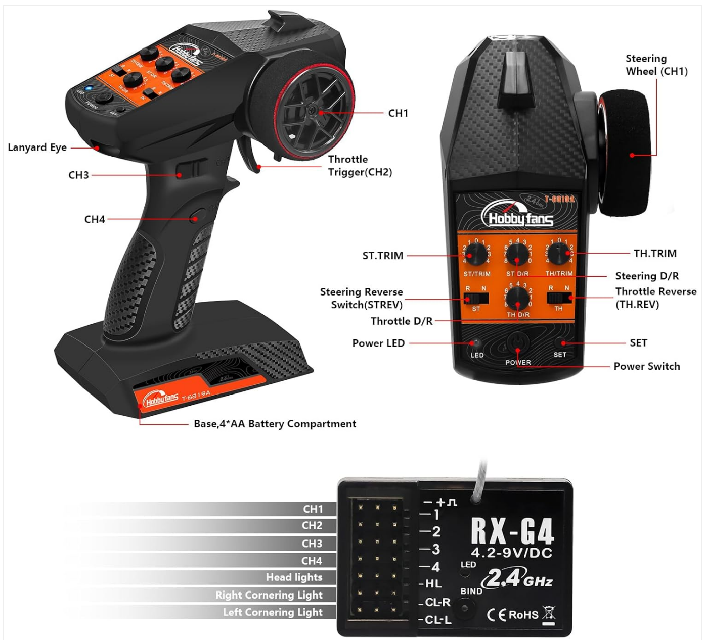
Figure 5: Location of Steering and Throttle D/R adjustments.
