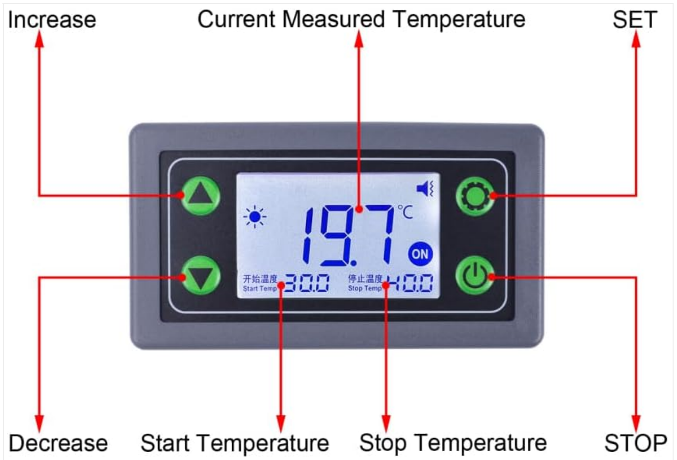
Figure 2.3: Detailed view of the display interface, showing the current measured temperature, along with the set start and stop temperatures for precise control.
