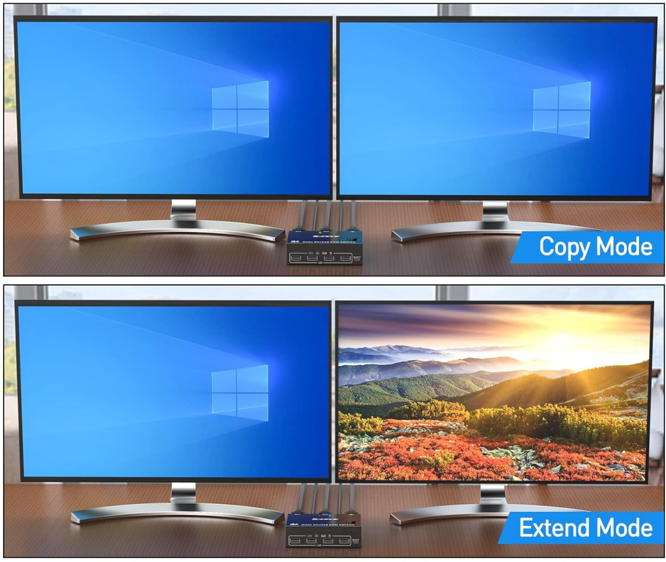
Image 5.2: Illustration of the two working modes: Copy Mode, where both screens show identical content, and Extend Mode, where the desktop is expanded across both screens.
